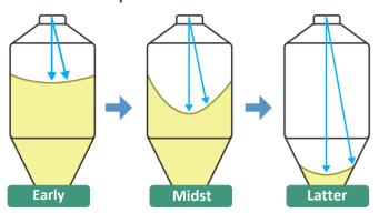
Accurately measure feed inventories even when full or with sinking mash feed
